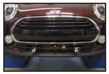
Hold the fascia as close to its original position, mark and trim the fascia around the convenience links and attachment tabs. Reinstall the washer reservoir and fascia.
