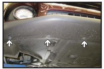
Using a 8MM socket, remove the seven (7) screws from the underside of the fascia.
