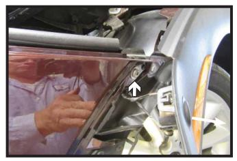
4. Pry the fender flare away from vehicle. Using a T30 Torx, remove the screw from behind the fender flare. Do this on both sides of the vehicle.
