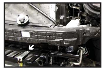
15. **Optional:** Attach the breakaway to the baseplate in the desired location with the supplied 1/4" hardware.
