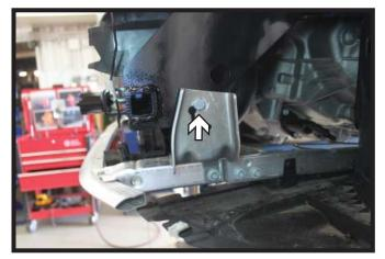
12. Reinstall the support bracket with the existing bolt. Mark the backside of the bracket where the existing hole in the baseplate hits. Remove the bracket and drill the hole with a 3/8" bit. Reinstall the bracket using the existing bolt and a 3/8"-16 x 1-1/4" bolt and lock nut. Do this on both sides of the vehicle. Fully tighten all hardware.
