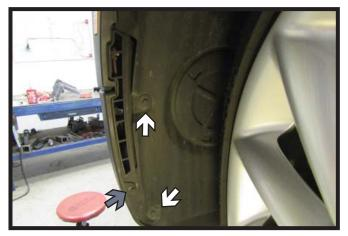
2. Using a 8MM socket, remove the two (2) screws (white) and one (1) push pin (gray) from the outer edge of the wheel well. Do this on both sides of the vehicle.
