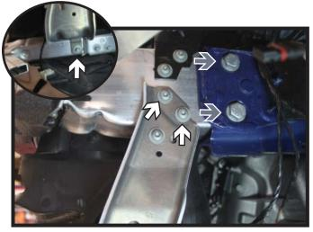
Using a T30 Torx, remove the two (2) screws from the top of the support bracket. Using a 8MM socket, remove the bolt from the bottom of the support bracket (inset). Set the bracket and 8MM bolt aside.
