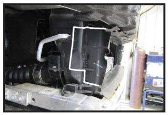
8. Trim the plastic shielding as shown on both sides of the vehicle for baseplate clearance.
