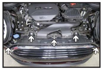
1. Using a T30 Torx, remove the five (5) screws from the top edge of the fascia.
