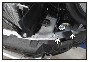
On the driver side, using a 10MM socket, remove screw from the upper horn and set aside (gray). Using a T30 Torx, remove the two (2) screws from the horn bracket (white). Disconnect all lines and set the horn assembly aside.
