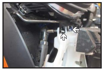
Using a T30 Torx, remove the two (2) screws from the washer reservoir. Disconnect/Plug all lines and set the reservoir aside.
