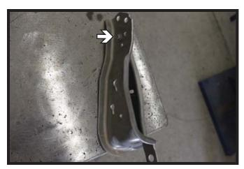
10. Remove the back strap from the support brackets by removing the T30 screw towards to top.
