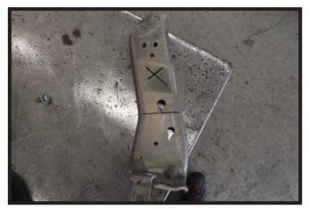
11. Trim off the upper section of the support brackets as shown.
